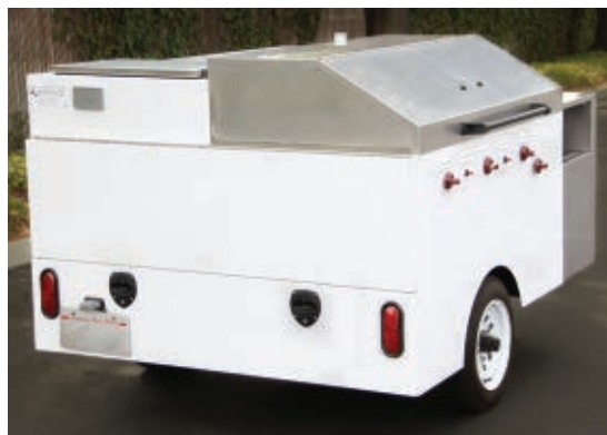
▲ FIGURE 2 This first-generation food preparation cart is 62 in. wide and 75 in. long, and the tongue, which connects to the tow vehicle, accounts for an additional 3 feet of length. The cart is designed to be towed to a destination, unhooked from the tow vehicle, and pushed onto a sidewalk for three-minute meals.
